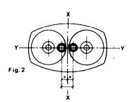
FOR SIMPLE SPINDLE ADJUSTMENT THE "X" "X" AND "Y AXIS OF THE COMPONENT SHOWN IN FIG. 1 SHOULD COIN CIDE WITH THE "X" ...X... AND ...Y... "Y" AXIS OF THE DRILL HEAD AND DRILLING UNIT AS SHOWN IN FIG SPINDLES SHOULD THEN BE ADJUSTED IN THE MANNER SHOWN IN FIGS 3 AND 4
